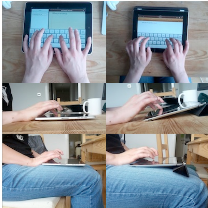
Figure 6.2. Typing on a tablet with (right) and without (left) a smart cover
